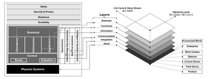
Figure 4: Industrial Internet of Things abstraction, functional domains, crosscutting functions and system characteristics
