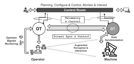
Figure 6: An illustrative example of Industrial collaboration between Operator and Machine for Training and Human-to-Machine interaction
